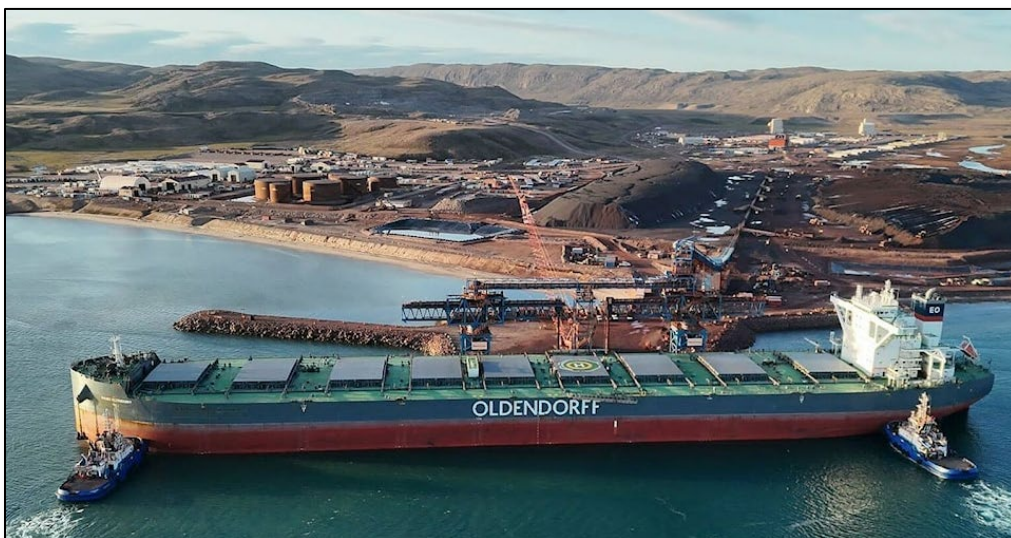
This Capesize ore ship is 300 metres long and 50 metres wide and is twice the size of other carriers used by Baffinland.
